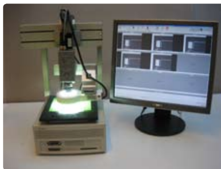
Scorpion Desktop AOI with Sony SmartCam and Robokid Desktop Robot
