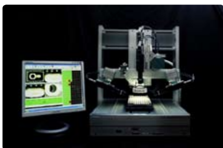
Sony desktop robot, firewire cameras and Scorpion Vision Software working together.
